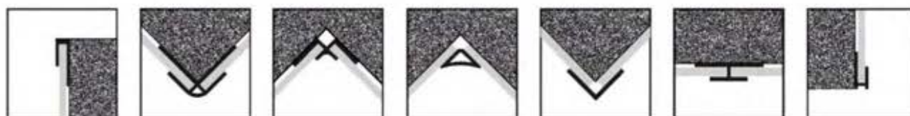
End External Corner Internal Corner Scotia Finishing L-Shape H Joint Base Seal
