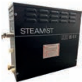
Steam Generator Top access for servicing 150mm left side clearance for Plumbing & Electrical
